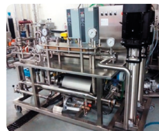
Membrane filtration system
